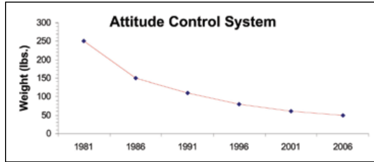
Figure 14. Relative weight of a spacecraft attitude control system for a fixed capability [9]
